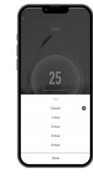
Using the Timer function, the heater can be set to turn off after a specified amount of time. Choose **Timer** at the bottom of the screen, select the duration of time that you want the heating to stay on for. The heater will turn off after the selected amount of time has passed.
