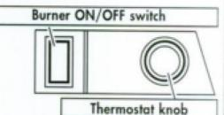
Start the machine acting on the apposite (ON/OFF) burner switch and wait for 30 sec. fto obtain the filling of the gasoil pump, act on the thermostat knob and put the temperature selector at 90° C for almost 30 sec. than, select tha water working temperature acting on the same knob.
