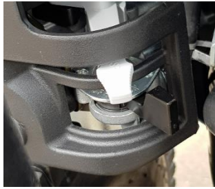
Fig5: Warm start or trouble start position - Engine Fuel tap lever (black) to the right and choke lever (grey) in centre position. Don't forget to move this choke lever immediately to the right (off position) when the engine starts running
