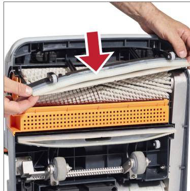
2. Check if dirt/debris are clogging the squeegee inlet and if the blades are worn or damaged.
