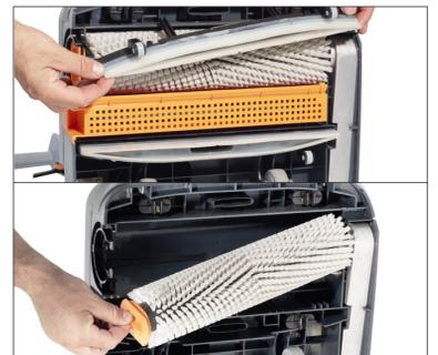
14. Remove the squeegee. Unscrew by turning the knob clockwise to remove the cylindrical brush.
