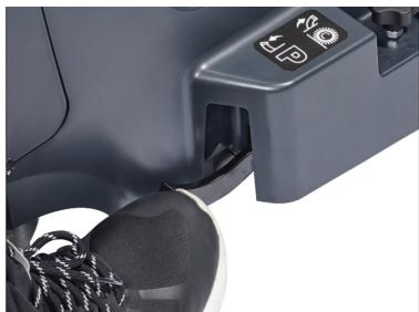
11. For the transportation and the parking of the machine, push down the pedal (slightly lift the front of the machine by tilting the handlebar).
