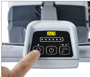
9. For double scrubbing, press the button to switch off the vacuum.
