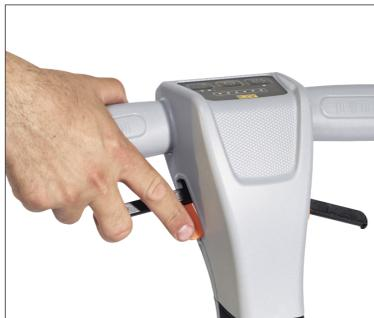
8. For sweeping functions, lift/lock the right lever to lift the front squeegee in order to collect light debris.
