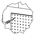
Screw panel to wall (minimum of 4 fixings)
