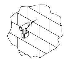
Drill holes to suit fixings. Check for pipes & cables first.
