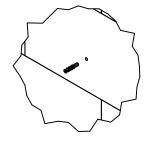
Fit wall fixing plugs (to suit wall type)
